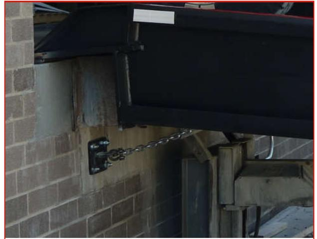
**CHAINS/BRACKETS**– Chains and brackets are provided on every dock-to-ground ramp. Once the brackets and chains are securely fastened to the face of the dock the ramp is ready for use.
