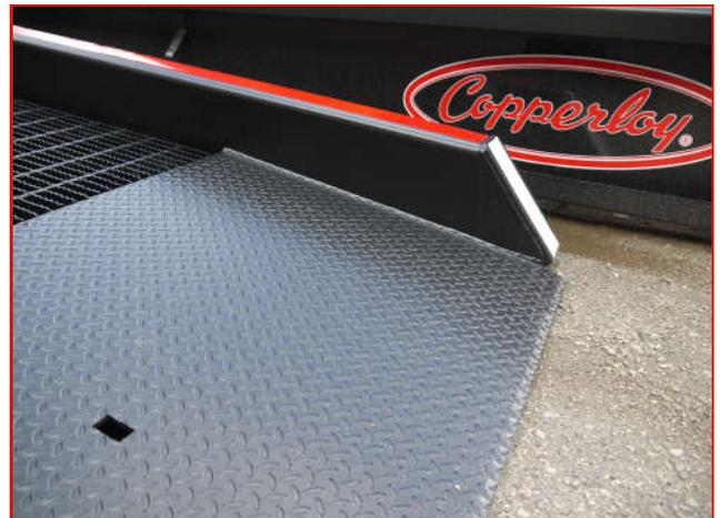
**LOW END PLATE** – 36" long. Approach plate is beveled from the underside to provide a smooth ground-level entry, eliminating jolts and bumps when forklifts travel on and off the ramp.
